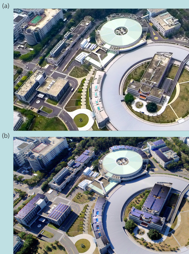
Fig. 1: Roof landscape (a) before and (b) after the installation of the PV systems.
